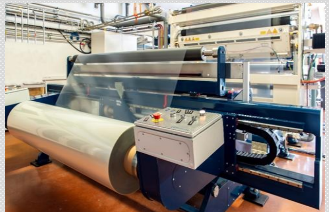
NORCOP's Plasma Station operates at atmospheric pressure and is capable of coating films with width up to 2000mm at speeds up to 100m/min.
